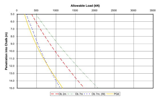
Figure 1 Low SPT profile: allowable bearing capacities for varying overburden conditions
